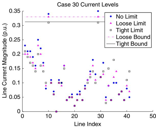
Fig. 4 30-bus line currents at no, tight, and loose limits
