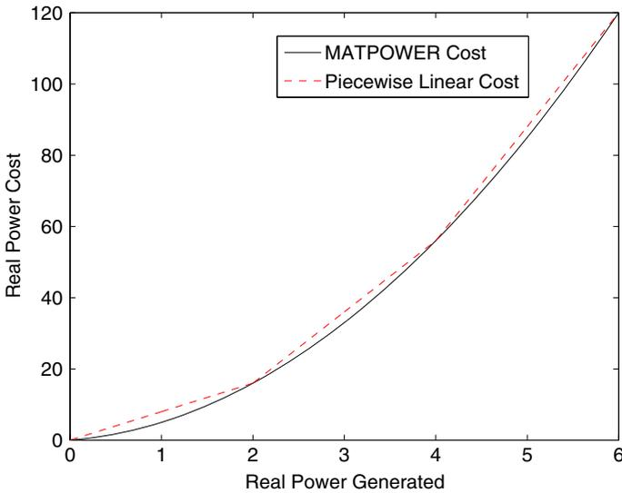
**Fig. 1** MATPOWER cost versus piecewise linear approximation cost
