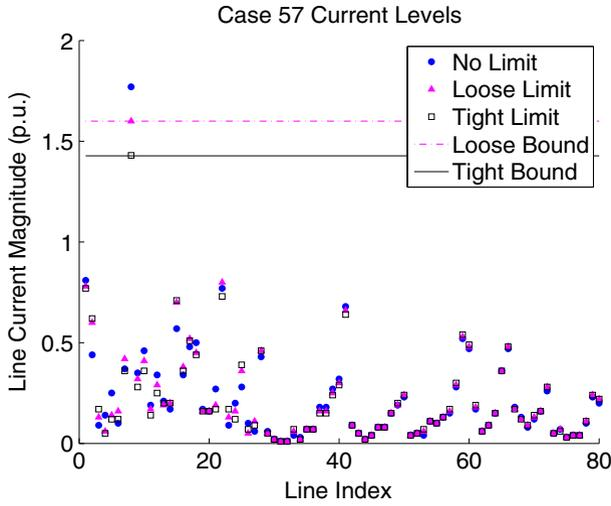
Fig. 5 57-bus line currents at no, tight, and loose limits
