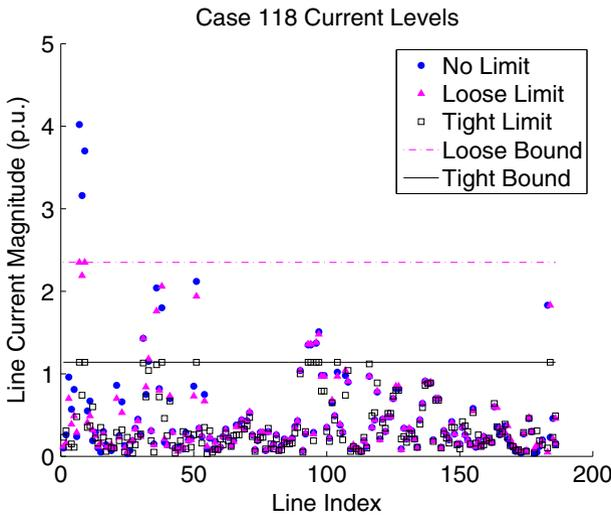
Fig. 6 118-bus line currents at no, tight, and loose limits
