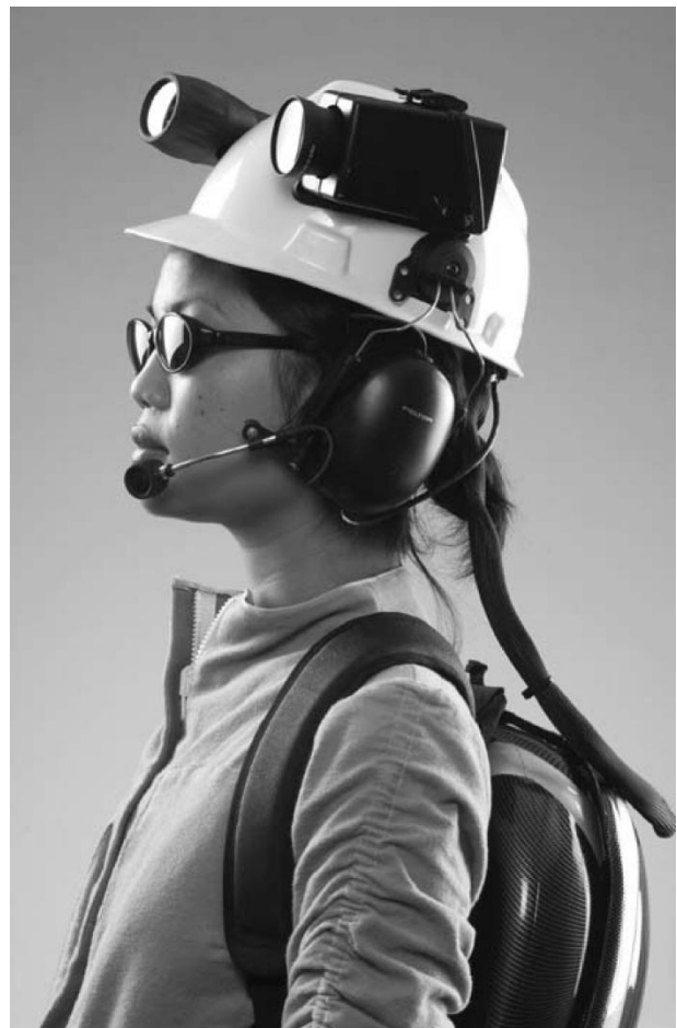
Fig. 3. The human tele-actor transmits images from the remote environment using the helmet-mounted video camera and responds to user votes. Helmet design by E. Paulos, C. Myers, and M. Fogarty. (Photo by B. Nagel.)
