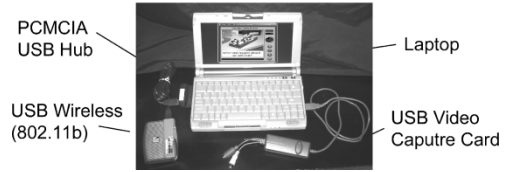
Fig. 8. Hardware configuration for the cameraperson. The hardware configuration of the tele-actor is similar but has a helmet-mounted camera.
