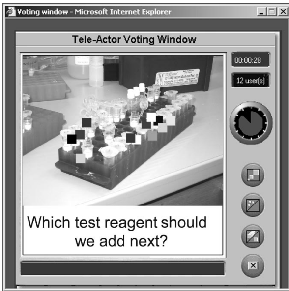
Fig. 1. The SDV interface as viewed by each user. In the remote environment, the tele-actor takes images with a digital camera which are transmitted over the network and displayed to all participants with a relevant question. With a mouse click, each user places a color-coded marker (a “vote” or voting element) on the image. Users view the position of all votes and can change their vote positions based on the group’s response. Vote positions are then processed to identify a “consensus region” in the voting image that is sent back to the tele-actor. In this manner, the group collaborates to guide the actions of the tele-actor.
