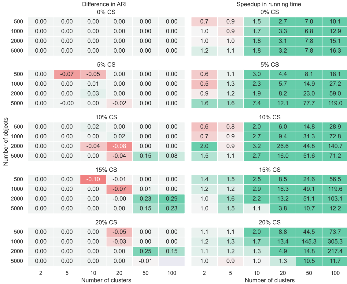
Figure 10: Comparison of baseline version PCCC with version PCCC-N5-S. The heatmaps on the left show the absolute difference in ARI (ARI of PCCC-N5-S minus ARI of PCCC) for the different instances and constraint set sizes, averaged across repetitions. The heatmaps on the right show the speedup (running time of PCCC divided by running time of PCCC-N5-S) of version PCCC-N5-S for the different instances and constraint set sizes. When the number of clusters is large (50 or more), the PCCC-N5-S version is considerably faster than the baseline version and delivers similar or substantially better ARI values.
