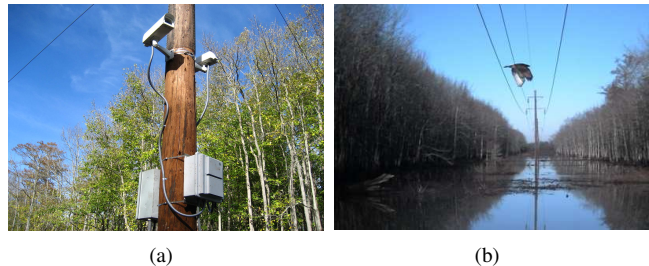
Fig. 1. Our autonomous observatory system installed along Bayou DeView, a bottomland forest near Brinkley, Arkansas. (a) The installation site. (b) A high resolution video frame of a red-tailed hawk captured by the system on Dec. 13, 2006. The red-tailed hawk has a body length of 22 inches and a wing span of 56 inches, close in size to the IBWO.
