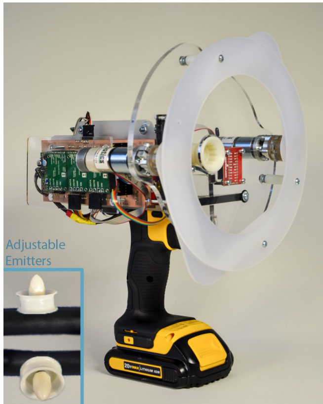
Fig. 1: The Device for Automatic Tuning of Emitters (DATE) can guide workers through fields to adjust passive irrigation emitters. The DATE features a novel two-stage manipulator that cages co-designed adjustable emitters (shown in inset).
