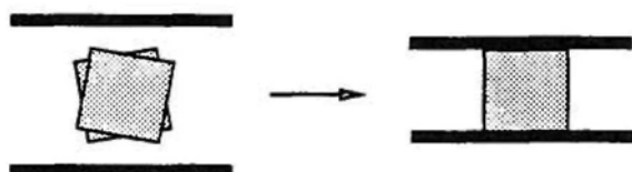
Figure 3.2: Top view of the parallel-jaw gripper grasping a part (shaded square). Small variations on the part's initial orientation are cancelled out during grasping so that the final orientation is guaranteed to be as shown on the right.
