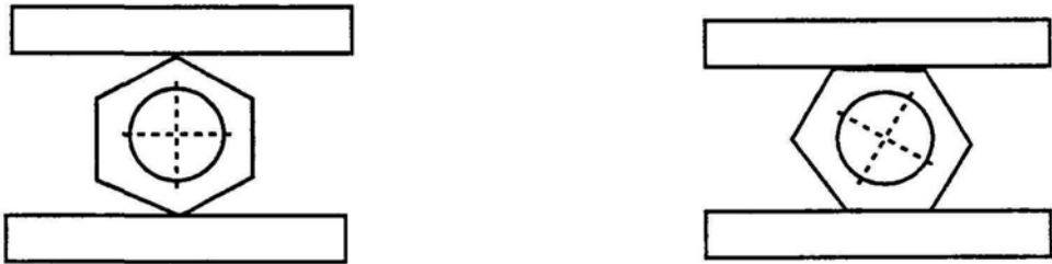
Figure B.2: Two-dimensional projection of a parallel-jaw gripper and a hex nut. The grasp on the right is stable in the sense that small perturbations in orientation produce restoring forces.
