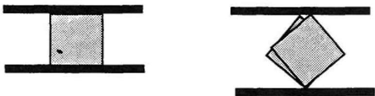
Figure 3.4: We define the configuration on the left as stable and the configurations on the right as wedged .
