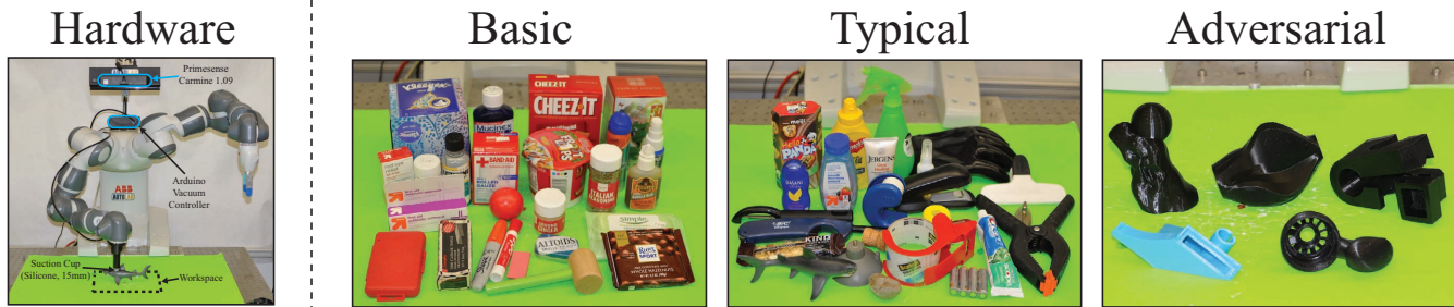
Fig. 5: (Left) The experimental setup with an ABB YuMi equipped with a suction gripper. (Right) The 55 objects used to evaluate suction grasping performance. The objects are divided into three categories to characterize performance: Basic (e.g. prismatic objects), Typical, and Adversarial.
