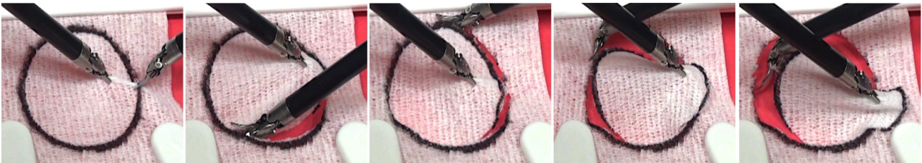
Fig. 4: Pattern Cutting of a 2D Orthotropic Tissue Phantom (2d-PCOTP). The finite state machine includes the following states: circle detection and estimation, warping, grasp OTP (push, grasp, retract), notch cutting (push, close, retract, twist), lower semicircle positioning, lower semicircle cutting, upper semicircle repositioning, upper semicircle cutting, active sensing for attachment detection (pull), and final cutting.
