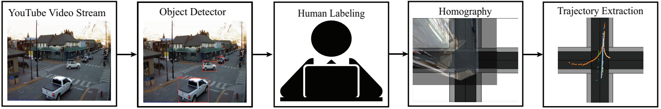
Fig. 2: TCP system architecture (excluding learning and analysis). First, we capture a video stream of a traffic intersection and use SSD, a deep object detection network, to identify and label vehicles. Then, we manually label the first detection of each vehicle in the video stream. Finally, we map the identified vehicles to a bird’s eye view using homography and run a probabilistic grouping algorithm to extract trajectories.
